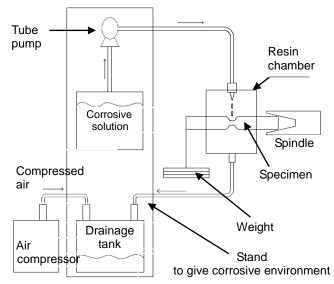
Fig. 7: Schematics of corrosion fatigue testing machine
