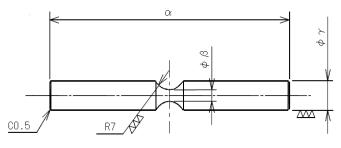
Fig. 3: The shape and dimensions of the specimen
